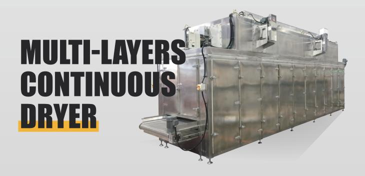
The continuous dryer of TSHS is divided into: the feeding section, the drying section, the hot air generating chamber, and the discharging section. We offer different planning and design according to the customer's product features (drying time, water content, and temperature) and available space for the equipment. The equipment meets the requirements of food hygiene regulations, and the parts exposed to food are made of stainless steel.
